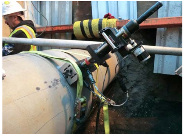
Fig. 11 Use straps for irregular shaped pipe sections, bends, or short sections
