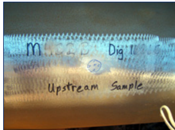
Fig. 8 Test locations with coating removed, SSM footprint area ground smooth, and test location polished
