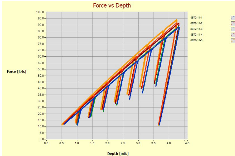
Fig. 10: Overlays of ABI force-depth data, true-stress versus true-plastic-strain curves, and yield strength calculation plots for Location 8BT2-11
