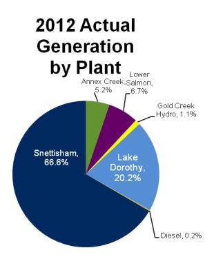
AEL&P's load is served with hydroelectric generation, but AEL&P also has backup diesel generation sufficient to serve the full load.
